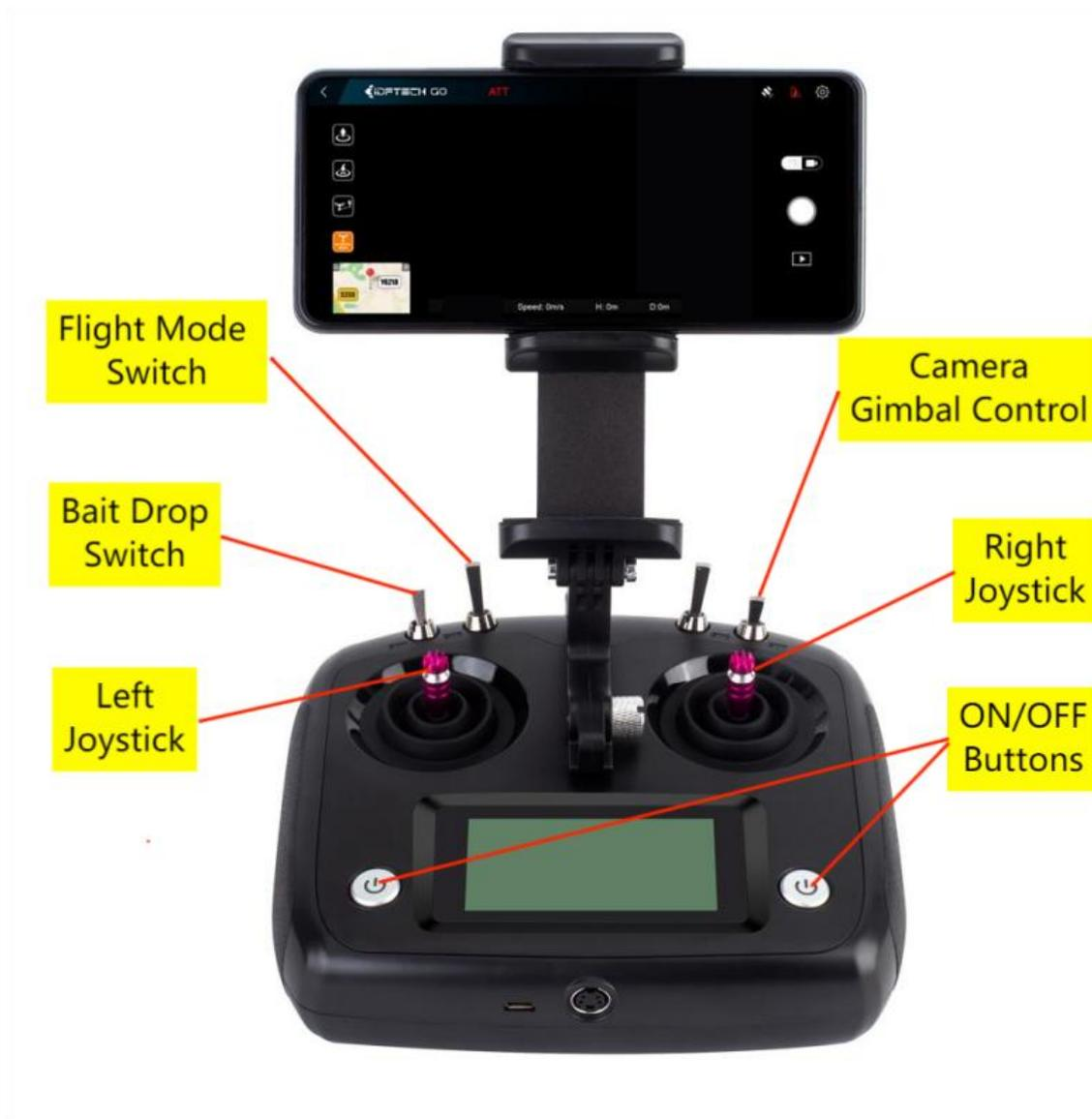
**Note:** When switching on the remote control, ensure the switches are set to the top position, otherwise the remote control will display a warning.
